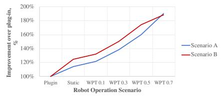
Fig. 11. Improvement on effective tasks per day at various robot charging scenarios vs plug-in charging
