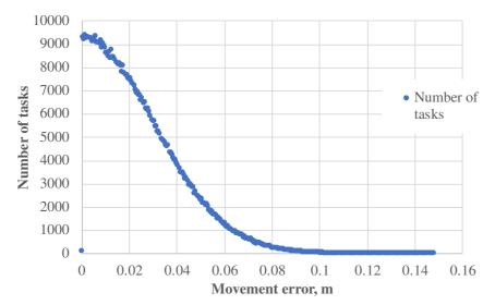
Fig. 6. Distribution of robot's movement precision over charging lines
