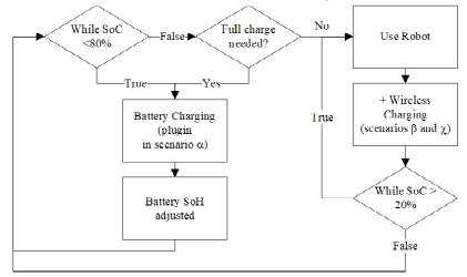
Fig. 5. General robot charging algorithms
