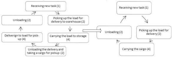
Fig. 2. Modes of robot operation for model's purposes
