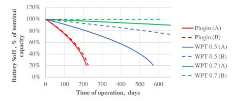
Fig. 8. Battery SoHat various robot charging scenarios
